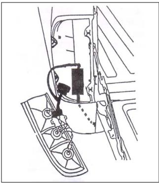
(g) Remove the old converter with harness from the taillight cavity.
