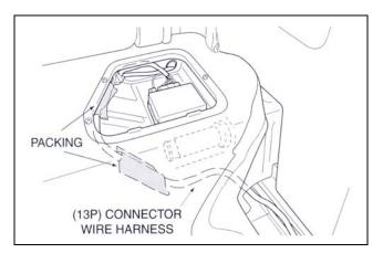
(8) Route the 13-Pin connector and secure with packing tape as shown.
