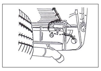
(f) Remove any foam or tie-wraps holding the converter harnesses to the taillight harnesses.
