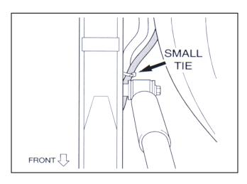
(d) Install a tie-wrap near the left rear shock as shown.
