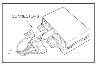
(4) Connect the 8-Pin and 2-Pin connectors of the converter box harness to the converter box.
