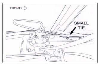
(c) Install a tie-wrap near the brake load-regulating valve.
