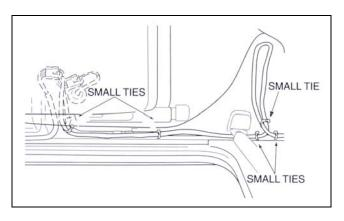
(10) Secure the converter box harness to the vehicle's harness using the 5 tiewraps as shown.
