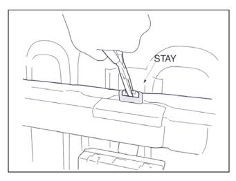
(5) Tighten the mounting bracket to the rear cab wall as shown.
