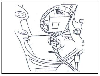
(m) Remove the old converter with harness from the taillight cavity.
