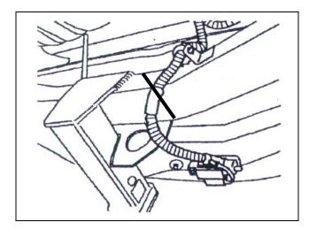
(c) Mount the new flat four-connector bracket to the hitch plate bracket using the original bolts.
