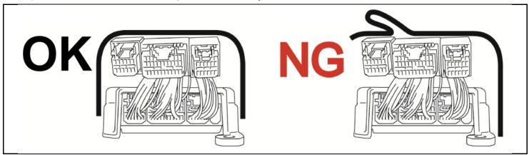
e) Pass a cable tie through the space under the airbag sensor, then connect another cable tie.
