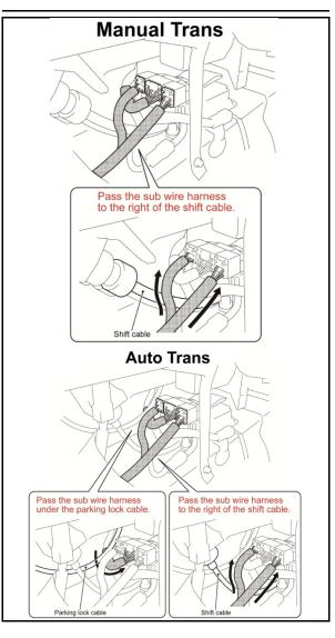
b) Connect the 3 vehicle-side connectors to the **NEW** sub harness. Reference the correct illustration based on transmission type for wire routing.
