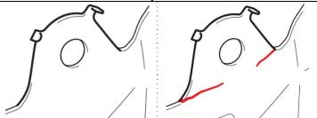
If the anchor is cracking but not separated or there are no cracks present, additional inspection is required. Complete **STEP 2** below then proceed to **SECTION X**.
