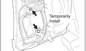
b) Temporarily install the 2 bolts that were removed with the seatbelt.
