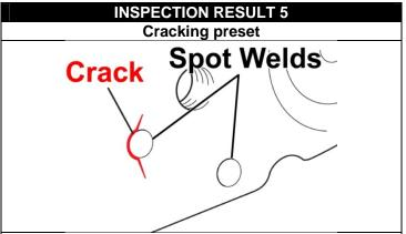
It is necessary to install the access panel reinforcement and replace the seat outer belt assembly. Complete **STEP 2** below then proceed to **SECTION XI.**
