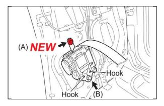
b) Position the seatbelt so that the hooks on the door panel engage with the holes on the seatbelt bracket and loosely install the bolts.
