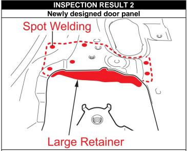
It is **NOT** necessary to install a reinforcement or replace the seat outer belt assembly because the door is already equipped with a large retainer. Proceed to **SECTION XII.**
