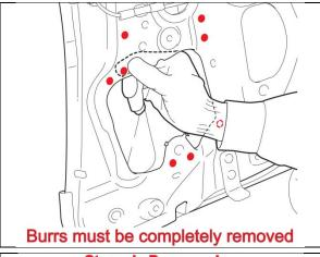
4) Confirm the burrs have been completely removed from the back side of the holes.
