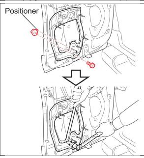
c) Install the nut plate and bolt. Hold the nut plate with a wrench (15mm) when tightening the bolt.
