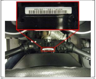
3. INSPECT THE LOT NUMBER ON THE SPIRAL CABLE NOTE: When viewing from the driver seat, the lot number will be upside down.
