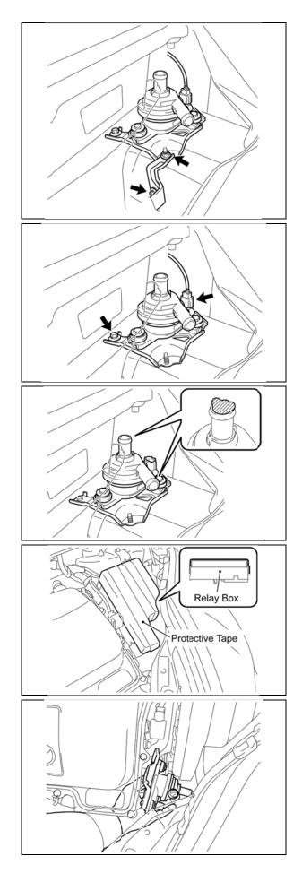
c) Remove the nut, bolt, and bracket.
