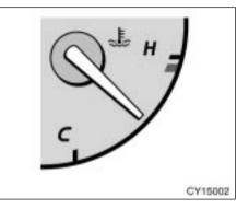
The gauge indicates the engine coolant temperature when the engine switch is on. The engine operating temperature will vary with changes in weather and engine load.
