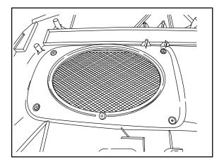
2. Install the NEW speaker grille and fasten in place using the push lock nuts provided in the repair kit.
