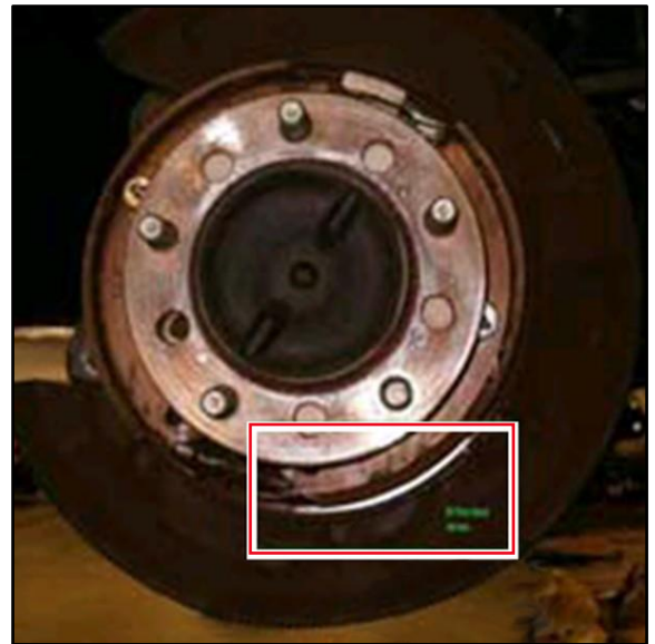
Figure 1. Example of Irregular Contact on Brake Plate
