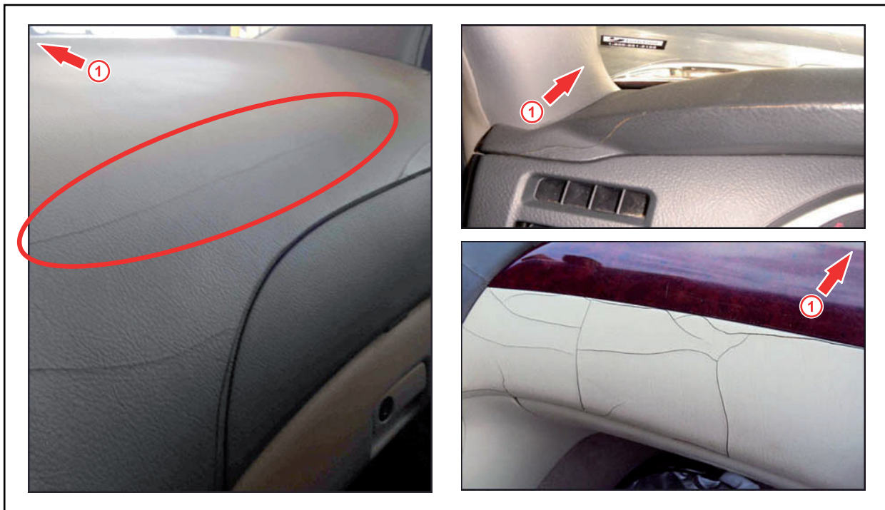
Figure 3. Examples of Cracked Condition
