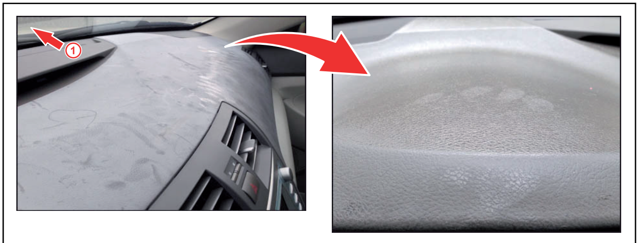
Figure 2. Example of Chalky Condition (Becomes Sticky in the Heat)
