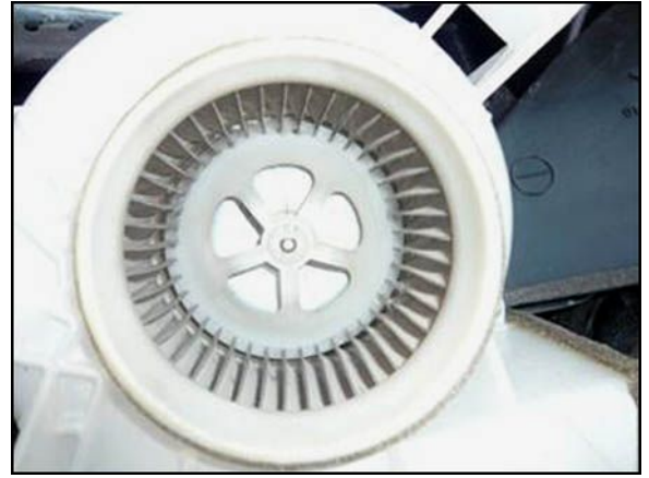
Figure 2. HV Battery Cooling Fan AFTER Cleaning
