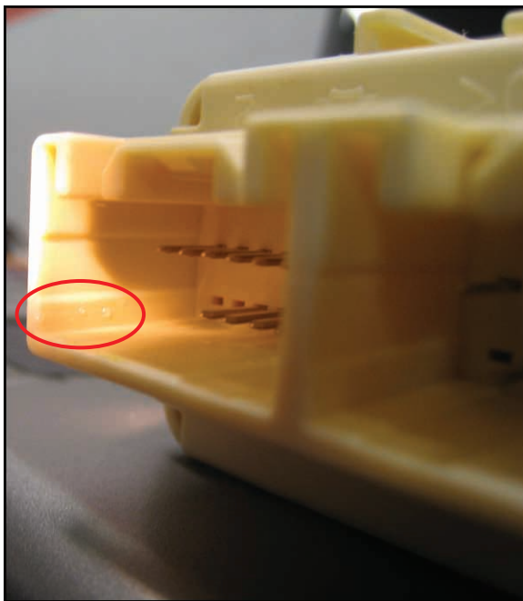
Figure 8. Liquid Droplets in Junction Block No. 1
