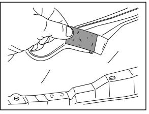
10. Perform the felt repair on both front corners of the moon roof structure.
